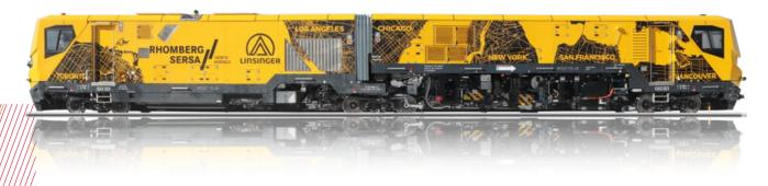
whomberg Sersa operates the latest LINSINGER SF02T-FS-LB milling machine with state of the any technology from the inventor of rail milling. This machine was specifically built to meet requirements of North American Transit Systems as well as to operate on Class 1 premises.
